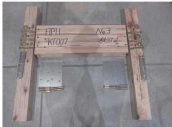
HP11-KTL007-3(カネシン)解体状況
