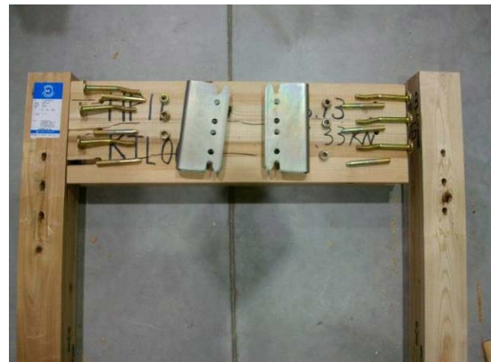
HP11-KTL007-13(タツミ)解体状況
