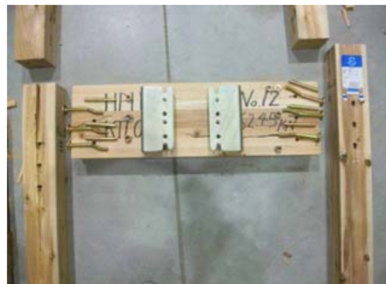
HP11-KTL007-12(タツミ)解体状況
